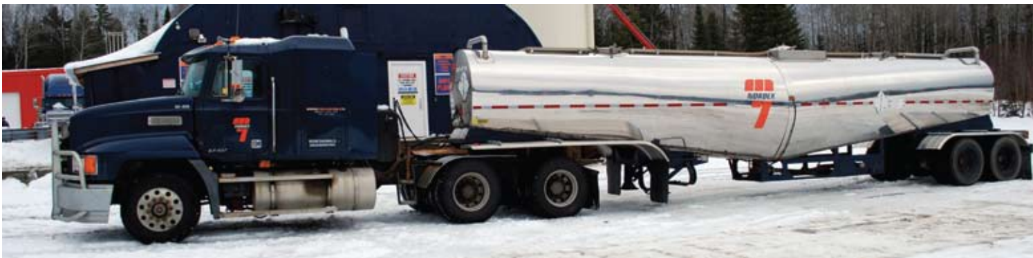
Nordex tanker truck used for transporting bulk emulsion explosives. The product is either transferred into specialized pumping units for underground use, or pumped into the drill holes in surface operations.
